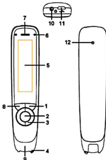
1. **Power On/Off & Back button:** Press 3 seconds to power device on or off. Press briefly to use as cancel function in the user interface
