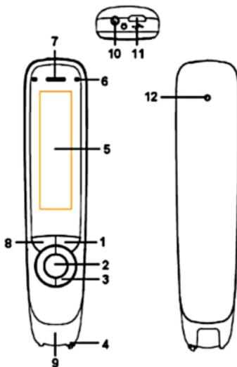
1. **Power On/Off & Back button:** Press 3 seconds to power device on or off. Press briefly to use as cancel function in the user interface
