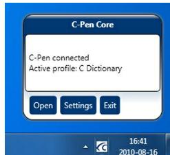
Connect the C-Pen to your computer using the included USB cable. To see the connection status, point the mouse cursor at the C-Pen tray icon to display the C-Pen Core status window.
