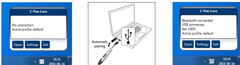
Connect the C-Pen to your computer via the included USB cable during the initial setup. The C-Pen Core software will automatically pair the C-Pen with your computer.
